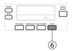
By using this function, you can delay the start of your washing programme by 30 minutes up to 23 hours.
